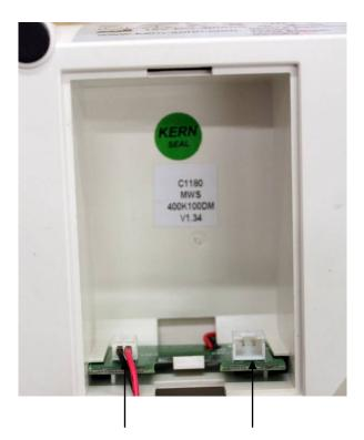
Connection **CN 4** for batteries (AA x 6)
