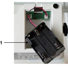
Carefully insert the rechargeable battery block and insert plug into connection CN 3
