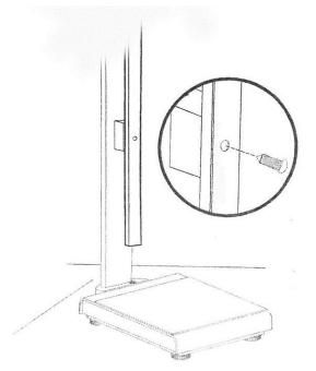
Extend the height measuring rod and tighten it in the lower hole of the bracket with the help of the appertaining screw.
