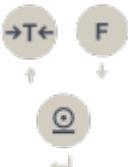
Press the tare key in the menu until UCAL 5 appears and confirm with the print key. Then use the tare key to advance to pos. 03 and confirm with the print key.
