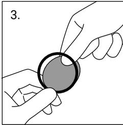
3. Now put me about a quarter of the way into the ring. Don't try to insert me completely into the ring straight away. That could damage my sensitive body.
