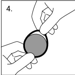
4. Now hold me between your thumb and forefinger and gradually pull me into the ring, always pulling up a small piece of the ring and letting me snap into place. Repeat this all around until I am completely in the ring.
