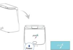
2. Put the Integrated Nucleic Acid Testing Device on a flat surface, connect the power supply, press the button on the front of the Instrument to start the warm-up process (power light flashes red). After about 2 minutes, warm-up is completed and the device is in standby (power light is blue).
