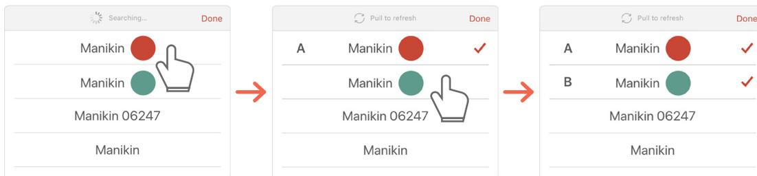
If there is a kit which is not calibrated among the kits, the calibration screen for the relevant kit will pop up immediately. You can connect manikins continuously after completing the calibration.
