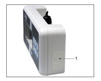
Open the battery compartment cover (1) at the base of the display unit and insert the rechargeable battery. Charge the rechargeable battery for at least 12 hours before initial use.
