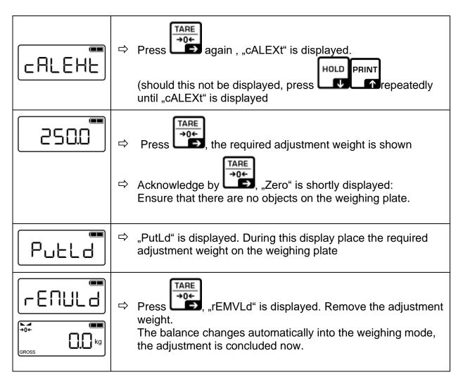
An adjusting error or incorrect adjustment weight will generate an error message ("WronG"), repeat the adjustment process.
