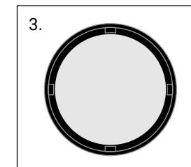
Place a new membrane into the ring so that it lays flat.
