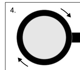
Tighten the ring and membrane onto the chest piece, so that they fit tightly.
