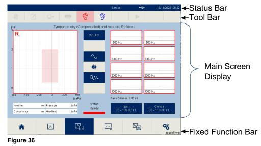
**Status Bar:** displays the Date/Time and the status of PC-connection  $\leftarrow$  (highlighted green if connected to PC-software (PC license must be activated) and MAICO Sessions is running).
