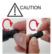
Never clean the probe tip while the tip is still attached to the probe
