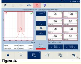
**NOTE**: A *Tympanometry* measurement is performed before each *Acoustic Reflex* test to find the maximum compliance pressure for better performance. However, it is possible to perform pure *Tympanometry* testing in this module if the *Acoustic Reflexes* are deactivated in the settings or on the screen (see section 5.6.10).
