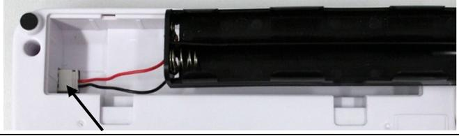
A photograph showing a black battery holder being connected to the metal contact point on the left side of the battery compartment. Red and black wires are attached to the holder, and an arrow points to the connection point. |
