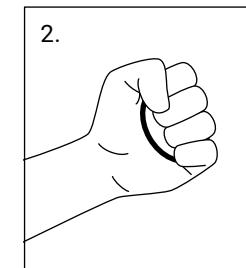
Take a matching ring and press it a few times in the palm of your hand. The movement and heat make the ring more flexible and assembly is easier.
