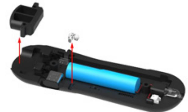
Now remove the circuit board from the housing.
