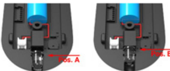
To change the battery, take the plug out of the connector and plug in a new battery using the same principle.
