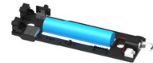
If you want to replace my LED, pull it out of the circuit board and insert the new one the same way. Please note that the longer contact is inserted into the opening on the right, as shown in the illustration.
