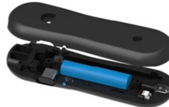
To get to the circuit board, you will need to remove the button and the indicator light.
